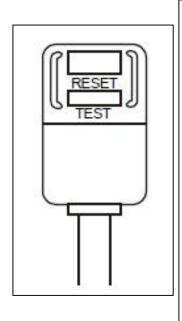
Your portable air conditioner is supplied with a Leakage-Current Detection and Interruption (LCDI) plug. This plug reduces the risk of fire due to arcing faults in the power supply cord. Please follow the instructions below to ensure that LCDI plug works properly.
